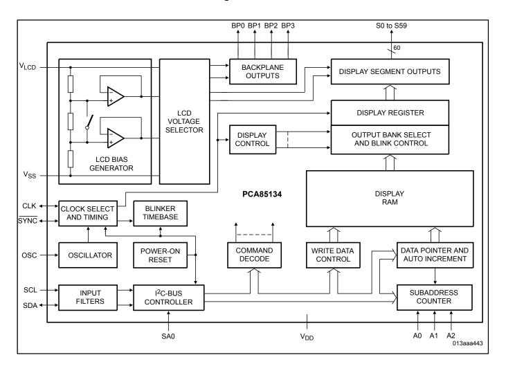
View additional information for Automotive 60 X 4 LCD Segment Driver for Multiplex Rates Up to 1-4.
