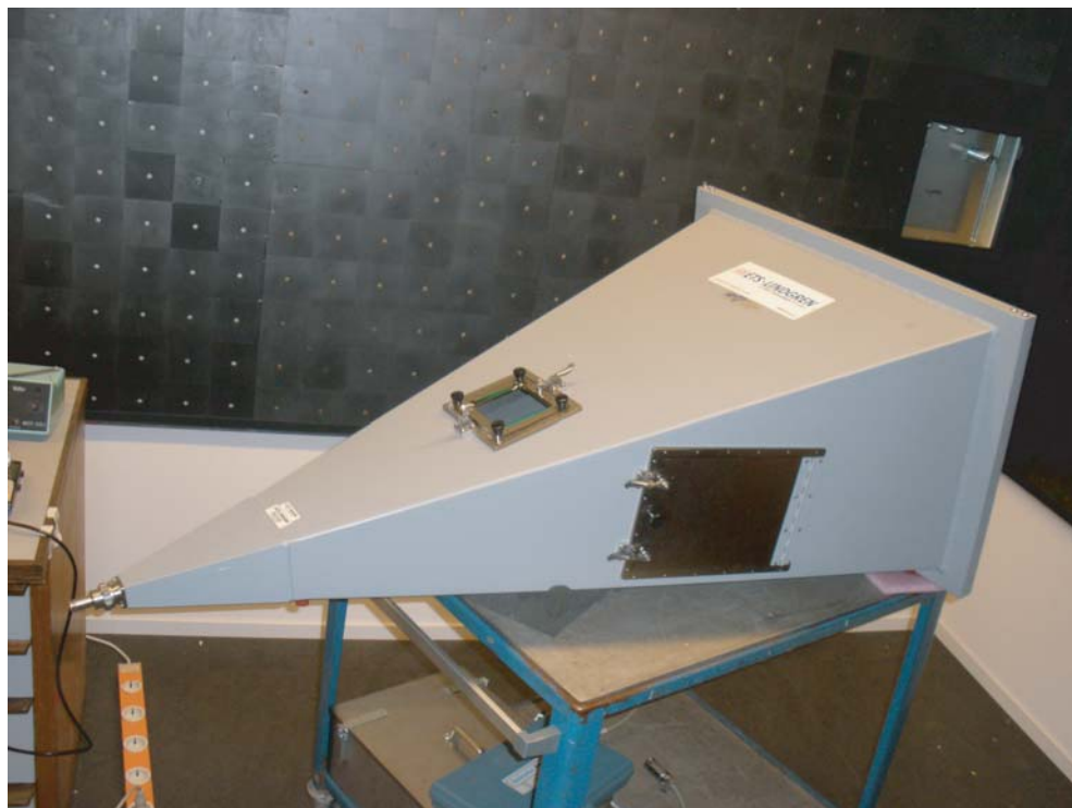
Fig 28. GTEM cell for immunity tests
