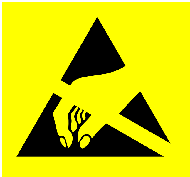
Fig 14. Warning label for an electrostatic sensitive device, denoting that the device is susceptible to damage
