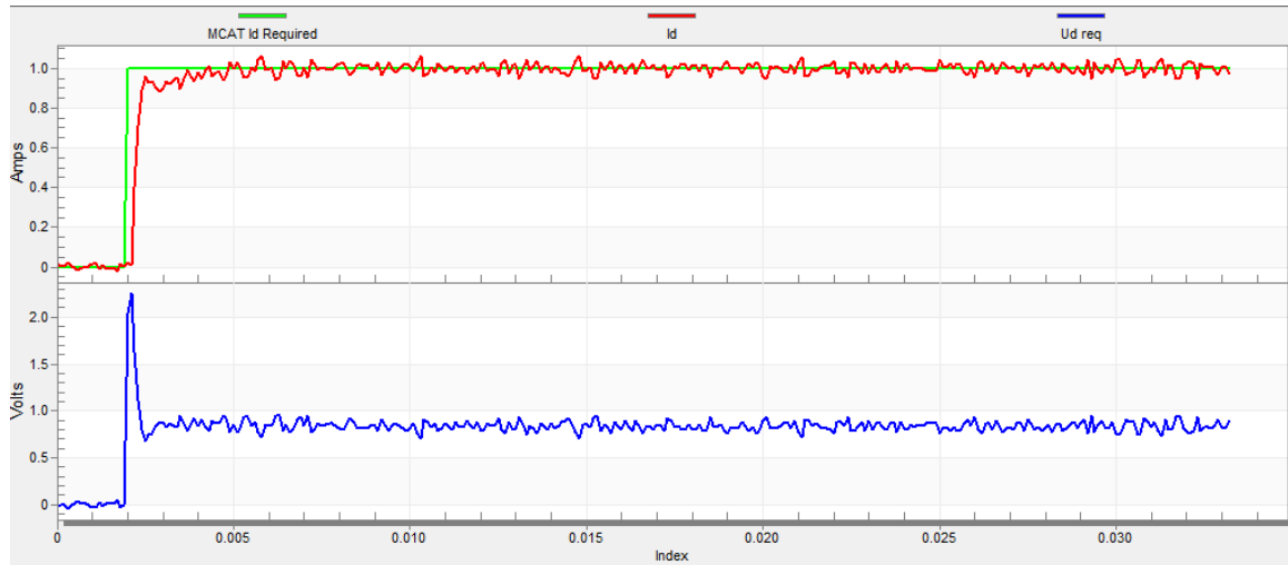
Figure 28. Optimal step response of the I_d current controller
