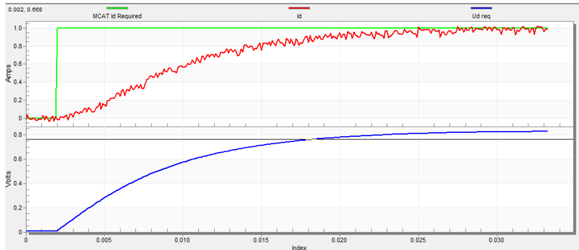
Figure 27. Slow step response of the I d current controller
