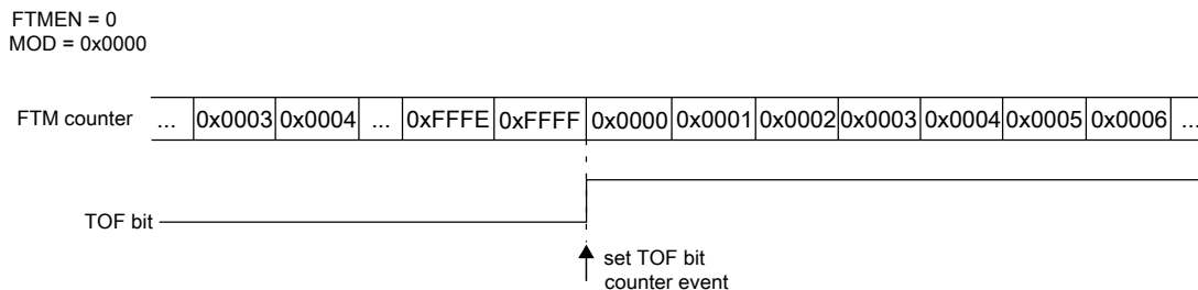
Figure 34-9. Example when the FTM counter is free running
